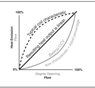
Desirable Equal Percent Flow and resulting heat output is achieved with linear results
