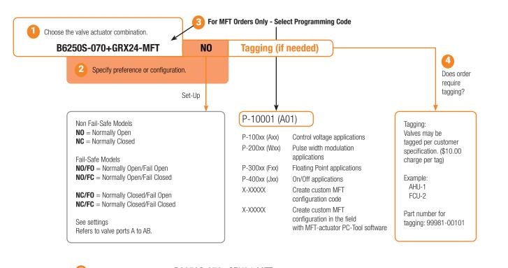
Complete Ordering Example: B6250S-070+GRX24-MFT Configuration: +N0 Programming: +A01 P10419 - 09/13 - Subject to change. © Belimo Aircontrols (USA), Inc.
