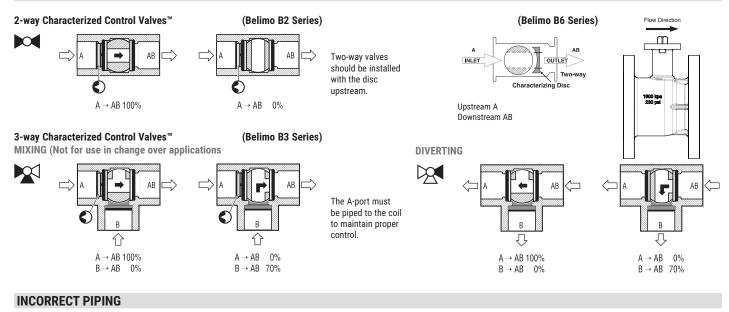
The A-port must be piped to the coil to maintain proper control.
