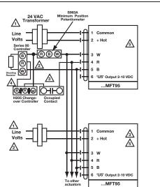
Wiring multiple actuators to a Series 90 controller using a minimum position potentiometer.
