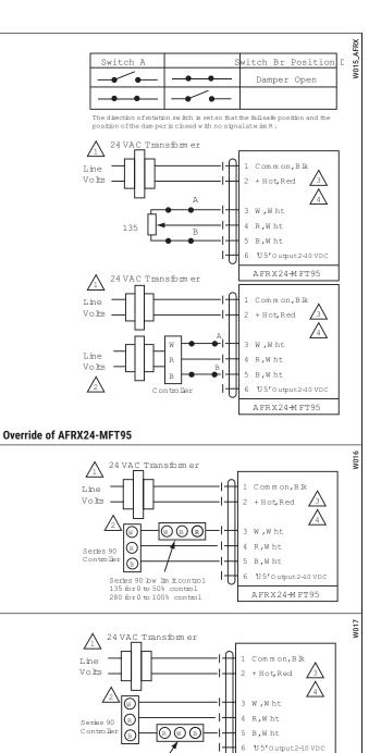
AFRX24-MFT95 used with a Series 90 controller and a Series 90 low limit control
